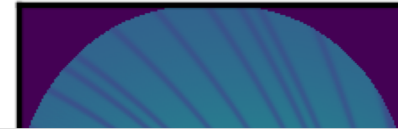
Combined Coverage LaB6 Det dist=220 mm, rot=30°; Energy=25keV
